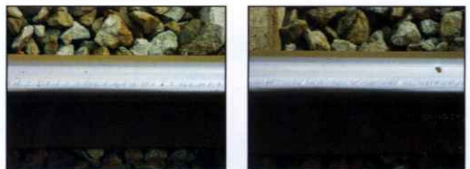
Fig. 2: Headchecks at gauge corner, widely spaced (left) and densely spaced with single ballast stone imprint (right)
