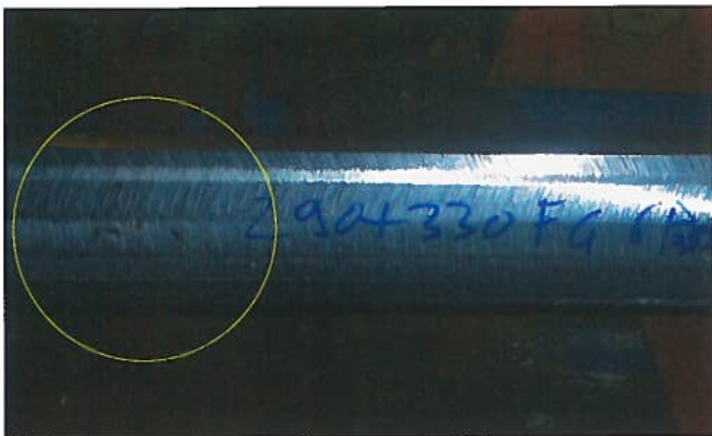
Fig. 9b: Squat removal – after 6 grinding passes
