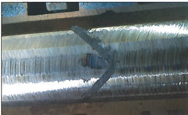
Fig. 6: Status following the removal of 6 mm of metal
