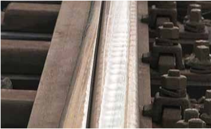
Above: Fig 3. Corrugation on a stock rail.
