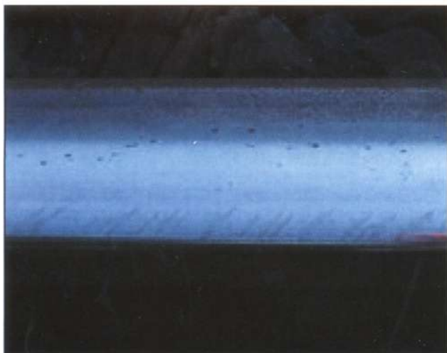
Fig. 4: Head checks in an early stage (left) and with beginning of material break-up (right)
