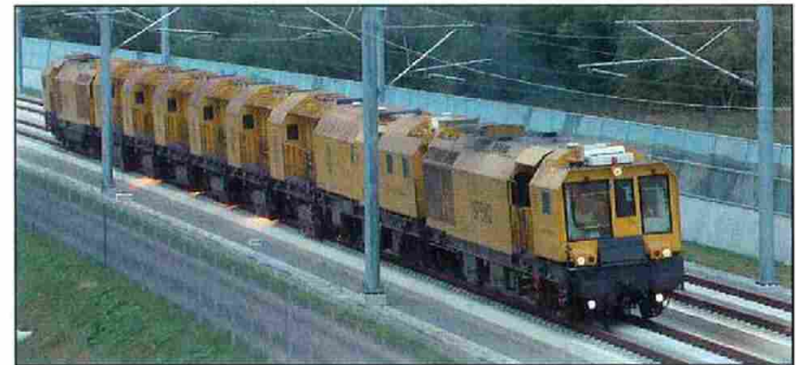
Fig. 6: The implementation of preventative rail grinding in The Netherlands has contributed to a significant reduction in the occurrence of RCF
