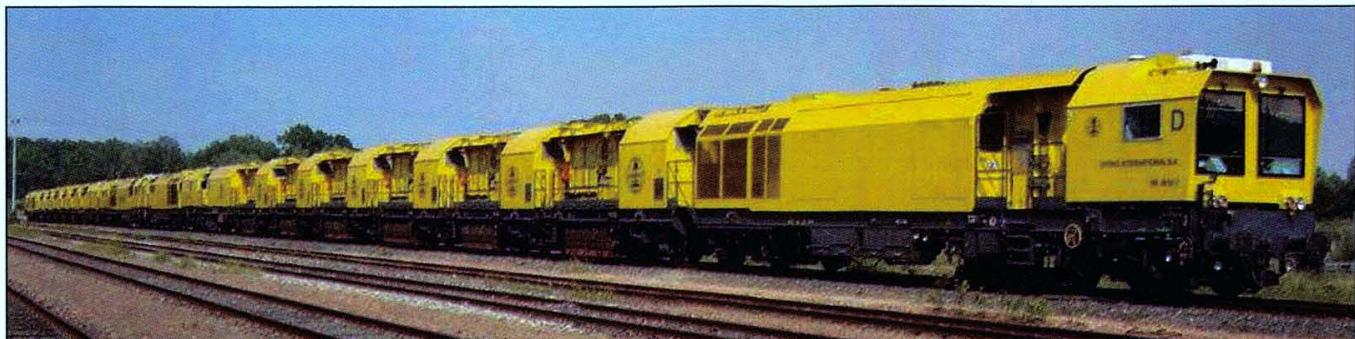
Fig. 5: The 96-stone grinding train that was used for one-pass grinding during the test campaign conducted in Germany
