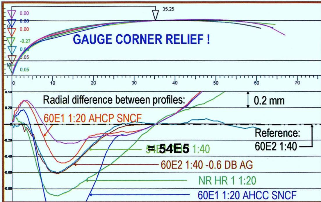
Fig. 4: Comparison of anti-headcheck profiles: the reference points are the centre of the rail head and 14 mm below at the gauge corner; the radial difference to the reference profile is shown at the bottom of the illustration (the reference profile is the 60E2 1:40 (bold line))
