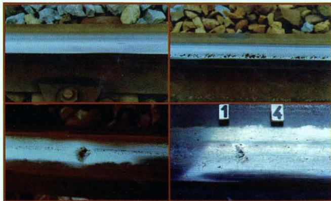
Fig. 2: Rolling contact fatigue (headchecks and squats)
