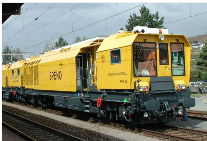
Figure 1. Modern rail grinding equipment, which is designed to fit within tight clearance envelopes, can produce the desired rail profile and surface condition in a single pass.
