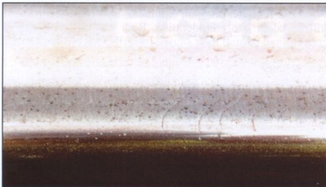
b: partly removed head checks, over which traffic has passed
