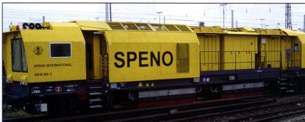
Speno's new 16-stone rail grinding train, the RR16 MS-2.
