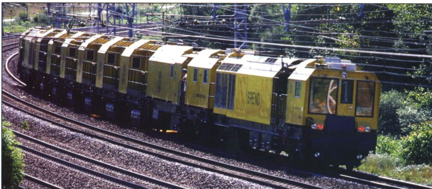
The RR 48 M-2 grinding train is dedicated for use by French National Railways.
