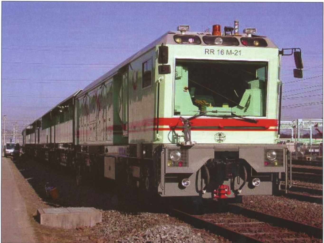
Fig. 1: Speno RR 16 M-21 and RR 16 M-22 grinding machines, coupled and synchronised to work together as a 32-stone grinding train
