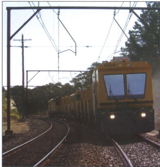
Fig. 1: Speno 48-stone rail grinding train working in the Sydney Metropolitan Region
