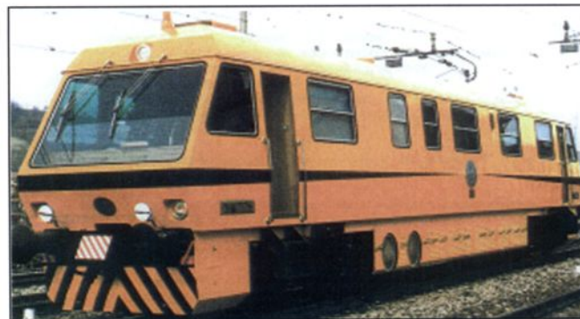
Fig. 23: Measuring and recording of rail surface defects
