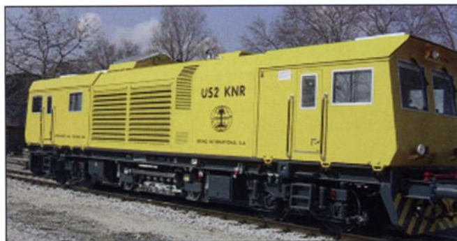
Fig. 22: Speno US2 ultrasonic rail testing car
