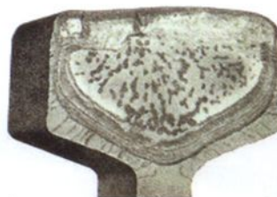
Fig. 1: Example of a kidney-shaped flaw or progressive transversal cracking, of internal origin
