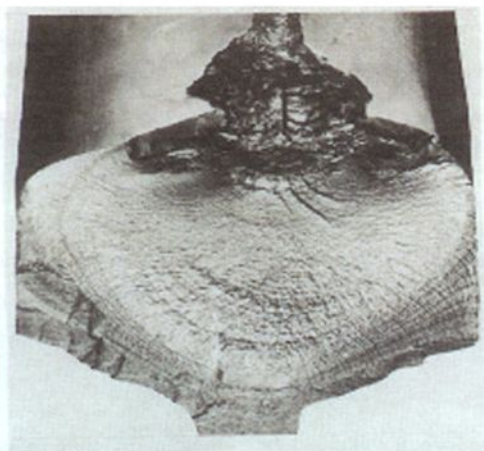
Fig. 6: Squat: cracking and local subsidence of the running surface
