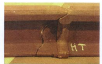
Fig. 2: Example of a weld breakage
